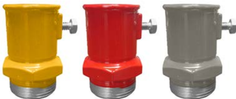
Frangible Coupling, 1.5" Thread (Part # FL-FC1.5) For 1" diameter riser, 1.5" thread for 1935 baseplate. Powder Coat Colors: Yellow (-Y), Red (-R), Marine Treated (-MT)
