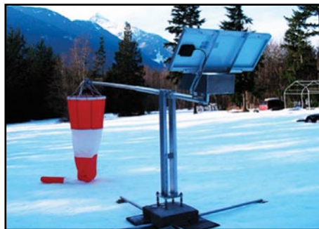
Tilt mechanism for easy, safe servicing by one person.
