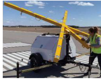
3. Tilt the light to the upright position
