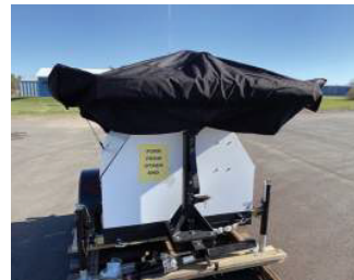
1. Fold "X" to stored position, apply cover
