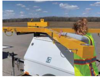
2. Extend the 4 light assembly arms
