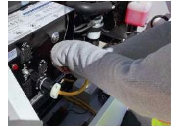
4. Start the generator and activate the lights
