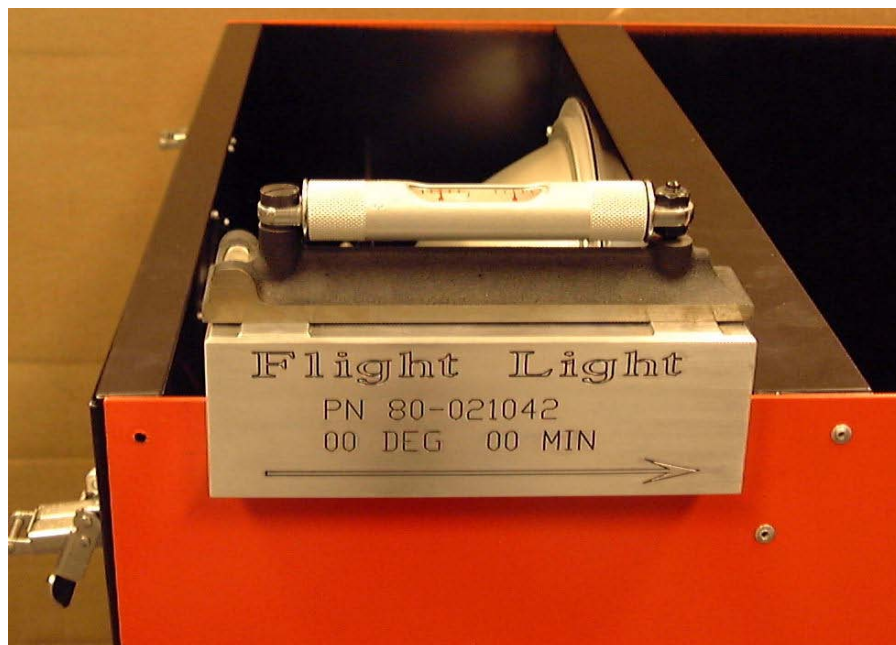
Figure 2 - Spirit level placed on aiming device.
