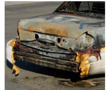
Police car destroyed from accidental combustion of pyrotechnic road flare.
