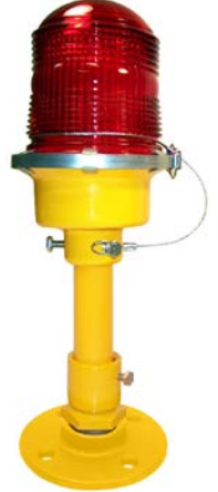
Shown with Riser, Frangible Coupling and Floor Flange (14" overall height)
