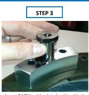
Insert 5/16" bushing into bushing block.
