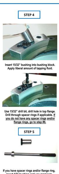
insert 1/2" bushing and use reamer to enlarge through holes in spacer rings and/or flange ring-ONLY. Use <u>depth gauge</u> to avoid reaming top flange hole- DO NOT REAM OUT top flange of base and/or top flange of extension or top section.
