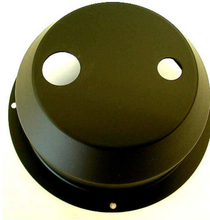
Fig. 17. SRA type bottom cover in good condition.
