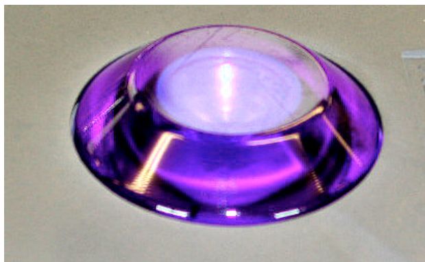
Fig. 3. ZA290 fitting. Close up of Prism, examine for dirt or damage.
