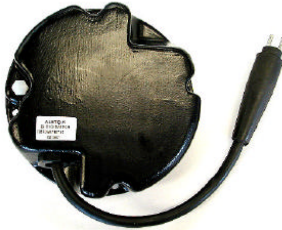
Fig. 12. external view of the bottom cover assembly in good condition.
