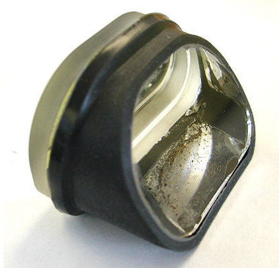
Fig. 7. Prism and gasket assembly.
