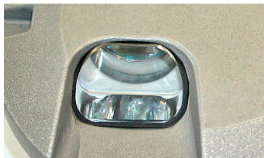
Fig. 2. Detail of prism in body assembly
