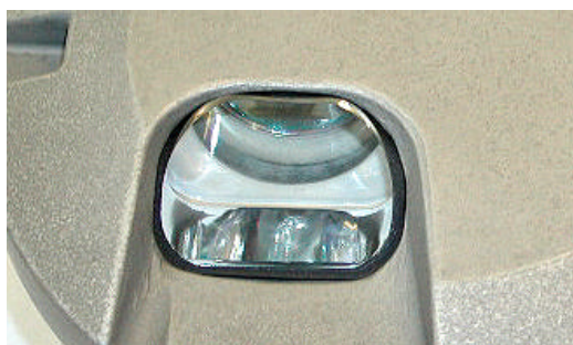
Fig. 2. Detail of prism in body assembly
