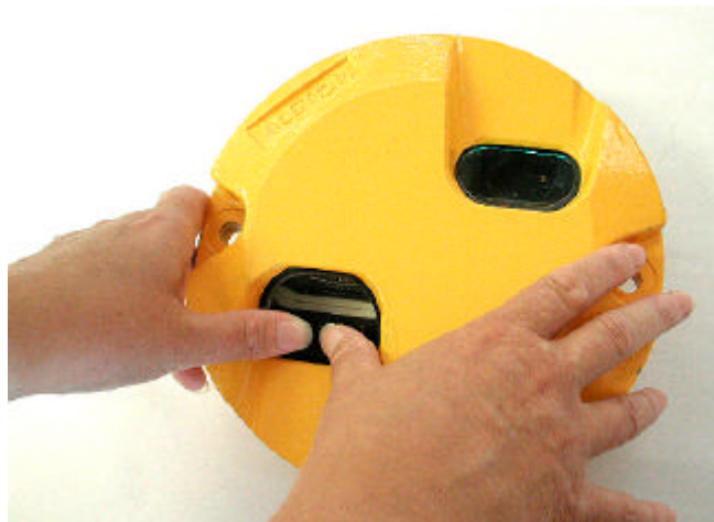
Fig. 6. Remove a prism by hand.
