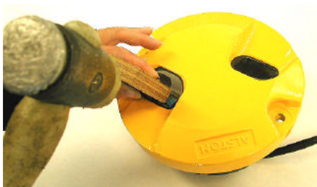
Fig. 7. Release a 'stuck' prism.
