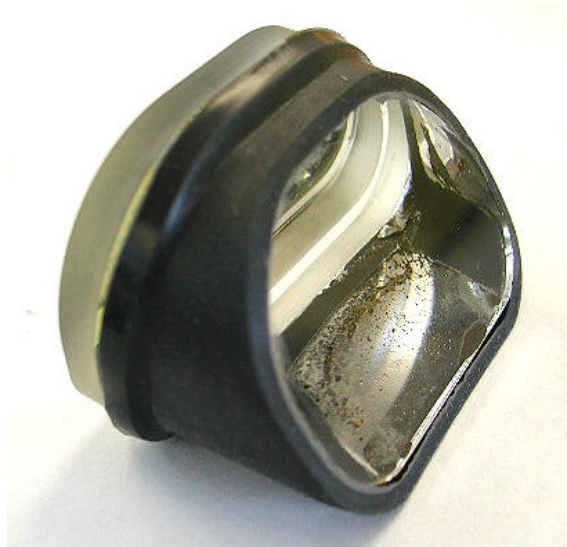
Fig. 8. Prism and gasket assembly.
